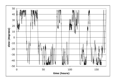
Figure 2: The slew history for one satellite in the best schedule generated. The horizontal axis is time; a total of one week. The vertical axis is the amount of cross-track slew necessary to execute the scheduled takeImages for this satellite. Note the preference for extreme slews. The extreme slews apparently minimize the total slewing time sufficiently to overcome the fitness pressure towards small slews.
