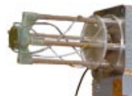
Figure 1: Photograph of the quadrifilar helical UHF antenna deployed on the Mars Odyssey spacecraft.
