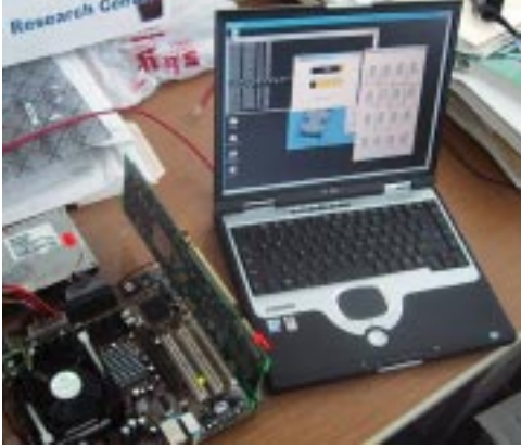
Figure 9: FPGA Fault Recovery demonstration system.
