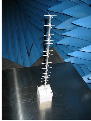
Figure 1: Computer graphics rendering of the best evolved antenna. It is 47 cm high, covers a 6 cm square footprint, and uses 1.587 mm radius wire. There are 15 crossed-elements.
